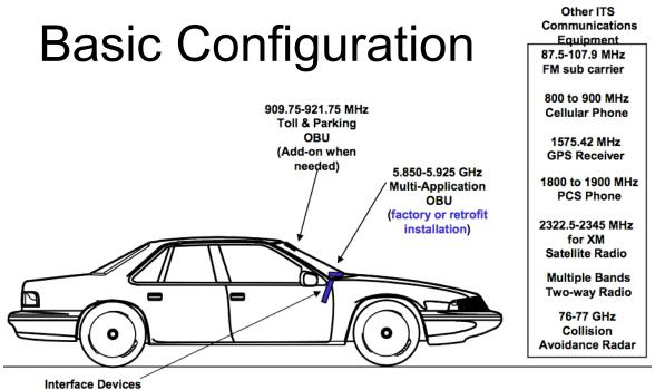
Interface Devices (Built-in Display, Annunciator, Microphone, Keypad, etc. connected to the Computer, (Cash, 2004) tota Bus)
